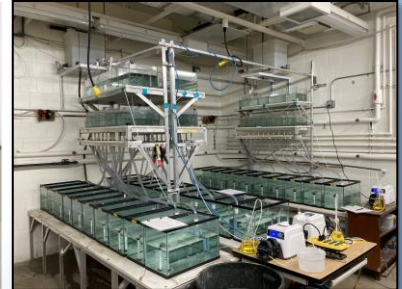
Replicated flow-through toxicity test system for comparative toxicity tests with target and nontarget animals
